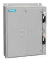
Duplex starter w/o alternator, Size 1 3/4, Three phase full voltage, Solid-state overload relay, OLR amp range 10-40A, 380-440/440-480V 50/60Hz coil, Combination type, Two 40A circuit breakers, Encl NEMA type 4X 304 S-Steel, Water/dust tight noncorrosive
