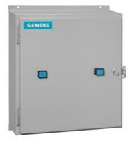
Duplex starter w/o alternator, Size 3, Three phase full voltage, Solid-state overload relay, OLR amp range 25-100A, 380-440/440-480V 50/60Hz coil, Non-combination type, Encl NEMA type 4X 304 S-Steel, Water/dust tight noncorrosive
