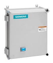
Non-reversing motor starter, Size 1, Three phase full voltage, Solid-state overload relay, OLR amp range 5.5-22A, 24VAC 50-60Hz coil, Non-combination type, Enclosure type 4X fiberglass, Water/dust tight noncorrosive, Standard width enclosure
