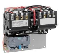
Reversing motor starter Size 0 Three phase full voltage Solid-state overload relay OLRelay amp range 0.75-3.4A 240VAC 50HZ / 277VAC 60HZ coil Non-combination type Enclosure type (open)
