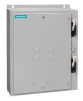
Duplex starter w/o alternator Size 3.5 Three phase full voltage Solid-state overload relay OLR amp range 50-200A 24VAC 50-60Hz Coil Combination type Two 200A disconnect switches Enclosure NEMA type 1 Indoor general purpose use
