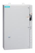
Non-reversing motor starter, Size 3, Three phase full voltage, Solid-state overload relay, OLR amp range 25-100A, 208VAC 60Hz coil, Combination type, 100A fusible disconnect, 100A/250V fuse clip, Encl NEMA type 4X 304 S-Steel, Water/dust tight noncorrosive, Standard width enclosure
