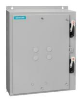
Duplex starter w/o alternator Size 1.75 Three phase full voltage Solid-state overload relay OLR amp range 10-40A 110VAC 50Hz / 120VAC 60Hz Coil Combination type Two 60A disconnect switches Enclosure NEMA type 4/12 Water/dust tight weather proof
