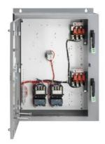
Duplex starter with alternator Size 1 Three phase full voltage Solid-state overload relay OLR amp range 3-12A 110VAC 50Hz / 120VAC 60Hz Coil Combination type Two 30A disconnect switches Encl NEMA type 4X 304 S. Steel Water/dust tight non-corrosive
