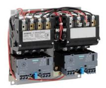
2-speed 3-phase motor starter Size 0 One winding consequent pole Constant horsepower Solid-state overload relays Low SPD OLR range 0.75-3.4A High SPD OLR range 3-12A 110V 50HZ / 120V 60HZ coil Enclosure NEMA type (open) No enclosure
