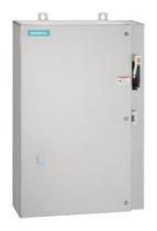
Non-reversing motor starter, Size 3, Three phase full voltage, Solid-state overload relay, OLR amp range 25-100A, Combination type, 100A fusible disconnect, 100A/600V fuse clip, Encl NEMA type 4X 304 S-Steel, Water/dust tight noncorrosive, Extra-wide enclosure
