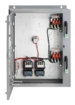
Duplex starter with alternator Size 1 Three phase full voltage Solid-state overload relay OLR amp range 0.25-1A 110VAC 50Hz / 120VAC 60Hz Coil Combination type Two 30A disconnect switches Encl NEMA type 4X 304 S. Steel Water/dust tight non-corrosive
