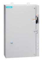
Non-reversing motor starter, Size 2, Three phase full voltage, Solid-state overload relay, OLR amp range 13-52A, 110V 50Hz / 120V 60Hz coil, Combination type, 60A non-fusible disconnect, Encl NEMA type 4X 304 S-Steel, Water/dust tight noncorrosive, Extra-wide enclosure
