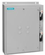
Duplex starter w/o alternator Size 2 Three phase full voltage Solid-state overload relay OLR amp range 13-52A 240VAC 50Hz / 277VAC 60Hz Coil Combination type Two 60A disconnect switches Enclosure NEMA type 1 Indoor general purpose use
