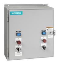
Duplex starter w/ alternator, Size 4, Three phase full voltage, Solid-state overload relay, OLR amp range 50-200A, 110V 50Hz / 120V 60Hz coil, Non-combination type, Enclosure NEMA type 1, Indoor general purpose use
