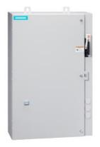
Non-reversing motor starter, Size 3, Three phase full voltage, Solid-state overload relay, OLR amp range 25-100A, Combination type, 100A non-fusible disconnect, Encl NEMA type 4X 304 S-Steel, Water/dust tight noncorrosive, Standard width enclosure
