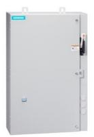
Reversing motor starter, Size 0, Three phase full voltage, Solid-state overload relay, OLR amp range 0.75-3.4A, 240V 50Hz / 277V 60Hz coil, Combination type, 30A disconnect switch, Encl NEMA type 4X 304 S-Steel, Water/dust tight noncorrosive
