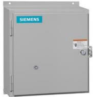
Reversing motor starter, Size 4, Three phase full voltage, Solid-state overload relay, OLR amp range 50-200A, 208VAC 60Hz coil, Non-combination type, Enclosure type 4X fiberglass, Water/dust tight noncorrosive, Standard width enclosure
