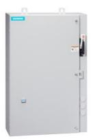
Non-reversing motor starter, Size 2 1/2, Three phase full voltage, Solid-state overload relay, OLR amp range 25-100A, 208VAC 60Hz coil, Combination type, 100A non-fusible disconnect, Encl NEMA type 4X 304 S-Steel, Water/dust tight noncorrosive, Standard width enclosure
