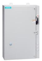
Non-reversing motor starter, Size 3, Three phase full voltage, Solid-state overload relay, OLR amp range 25-100A, Combination type, 125A circuit breaker, Encl NEMA type 4X 304 S-Steel, Water/dust tight noncorrosive, Standard width enclosure
