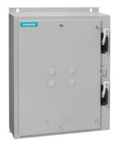
Duplex starter w/o alternator Size 4 Three phase full voltage Solid-state overload relay OLR amp range 50-200A Combination type Two 200A disconnect switches Encl NEMA type 4 painted steel Water/dust tight weather proof
