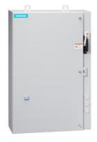
Reversing motor starter, Size 4, Three phase full voltage, Solid-state overload relay, OLR amp range 50-200A, 110V 50Hz / 120V 60Hz coil, Combination type, 200A disconnect switch, Enclosure NEMA type 4/12, Water/dust tight for outdoors
