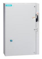
Non-reversing motor starter, Size 2 1/2, Three phase full voltage, Solid-state overload relay, OLR amp range 25-100A, 208VAC 60Hz coil, Combination type, 60A fusible disconnect, 60A/600V fuse clip, Enclosure NEMA type 1, Indoor general purpose use, Extra-wide enclosure
