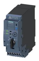
SIRIUS Compact load feeder DOL starter 690 V 24 V AC/DC 50...60 Hz 8...32 A IP20 Connection main circuit: plug-in, without terminals Connection auxiliary circuit: screw terminal
