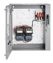
2-speed 3-phase motor starter, Size 0, One winding consequent pole, Constant or variable torque, Solid-state overload relays, Low Spd OLR range 0.75-3.4A, High Spd OLR range 3-12A, 110V 50Hz / 120V 60Hz coil, Combination type, 30A disconnect switch, Enclosure NEMA type 1, Indoor general purpose use
