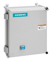
Non-reversing motor starter, Size 0, Three phase full voltage, Solid-state overload relay, OLR amp range 0.75-3.4A, Non-combination type, Enclosure type 4X fiberglass, Water/dust tight noncorrosive, Standard width enclosure
