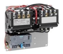
Reversing motor starter Size 1 Three phase full voltage Solid-state overload relay OLRelay amp range 0.25-1A 240VAC 50HZ / 277VAC 60HZ coil Non-combination type Enclosure type (open)
