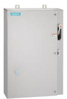
Non-reversing motor starter, Size 4, Three phase full voltage, Solid-state overload relay, OLR amp range 50-200A, Combination type, 150A circuit breaker, Encl NEMA type 4X 304 S-Steel, Water/dust tight noncorrosive, Standard width enclosure
