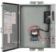
Pump control panel, Size 1, Three phase full voltage, Solid-state overload relay, OLR amp range 3-12A, 380-440/440-480V 50/60Hz coil, Standard type contactor, 10A circuit breaker, HOA Sel Sw. <(>&<)> Start P.B., Enclosure NEMA type 3/3R, Weather proof outdoor use
