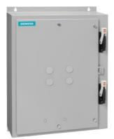
Duplex starter w/ alternator, Size 0, Three phase full voltage, Solid-state overload relay, OLR amp range 0.25-1A, 110V 50Hz / 120V 60Hz coil, Combination type, Two 3A circuit breakers, Enc NEMA type 4 painted steel, Water/dust tight for outdoors
