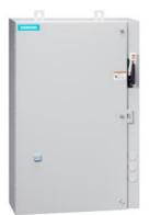
Non-reversing motor starter, Size 1, Three phase full voltage, Solid-state overload relay, OLR amp range 5.5-22A, 110V 50Hz / 120V 60Hz coil, Combination type, 30A fusible disconnect, 30A/600V fuse clip, Encl NEMA type 4X 304 S-Steel, Water/dust tight noncorrosive, Extra-wide enclosure
