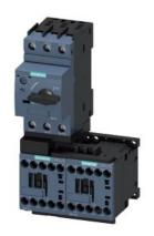
FUSELESS MOTOR STARTER REVERSING OPERATION 600V AC SZ S00 1.1-1.6A 220/240V AC 50/60HZ SCREW CONNECTION FOR SCREW MOUNTING OR 35 MM RAIL-MOUNTING TYPE OF COORDINATION 2 IQ = 150 KA ALSO FULFILLS TYPE OF COORDINATION 1 1NC (PER CONTACTOR)
