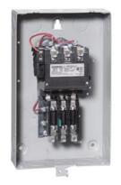
Non-reversing motor starter, Size 2 1/2, Three phase full voltage, Amb. compensate bimetal OLR, Contactor amp rating 60A, 24VDC coil, Noncombination type, Enclosure type 1, Indoor general purpose use
