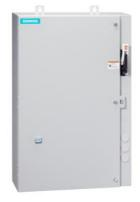
Non-reversing motor starter Size 3 Three phase full voltage Solid-state overload relay OLRelay amp range 25-100A 24Vdc coil Combination type 100A non-fusible disconnect Enclosure NEMA type 4/12 Water/dust tight weather proof Extra-wide enclosure
