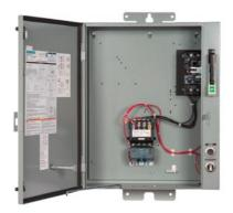
Pump control panel, Size 1, Three phase full voltage, Solid-state overload relay, OLR amp range 0.75-3.4A, 110-120/220-240VAC 60Hz coil, Standard type contactor, 3A circuit breaker, HOA Sel Sw. <(>&<)> Start P.B., Enclosure NEMA type 3/3R, Weather proof outdoor use
