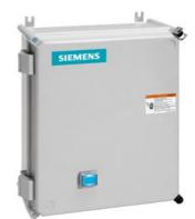
Non-reversing motor starter, Size 1, Three phase full voltage, Solid-state overload relay, OLR amp range 0.75-3.4A, 208VAC 60Hz coil, Non-combination type, Enclosure type 4X fiberglass, Water/dust tight noncorrosive, Standard width enclosure
