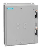
Duplex starter w/o alternator Size 4 Three phase full voltage Solid-state overload relay OLR amp range 50-200A 240VAC 50Hz / 277VAC 60Hz Coil Combination type Two 200A disconnect switches Enclosure NEMA type 1 Indoor general purpose use
