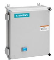
Non-reversing motor starter, Size 1, Three phase full voltage, Solid-state overload relay, OLR amp range 3-12A, 110V 50Hz / 120V 60Hz coil, Non-combination type, Enclosure type 4X fiberglass, Water/dust tight noncorrosive, Standard width enclosure
