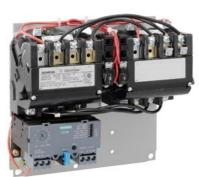
Reversing motor starter Size 1 Three phase full voltage Solid-state overload relay OLRelay amp range 3-12A 110VAC 50HZ / 120VAC 60HZ coil Non-combination type Enclosure type (open)
