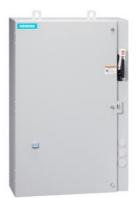
Non-reversing motor starter Size 0 Three phase full voltage Solid-state overload relay OLRelay amp range 3-12A 110-120/220-240VAC 60HZ coil Combination type 10Amp circuit breaker Encl NEMA type 4X 316 S-steel Water/dust tight noncorrosive Extra-wide enclosure
