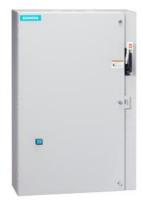
Reversing motor starter, Size 4, Three phase full voltage, Solid-state overload relay, OLR amp range 50-200A, 110V 50Hz / 120V 60Hz coil, Combination type, 150A circuit breaker, Enclosure NEMA type 1, Indoor general purpose use
