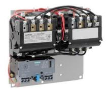
Reversing motor starter Size 1 Three phase full voltage Solid-state overload relay OLRelay amp range 0.75-3.4A 110VAC 50HZ / 120VAC 60HZ coil Noncombination type Enclosure type (open)
