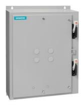
Duplex starter w/o alternator Size 1 Three phase full voltage Solid-state overload relay OLR amp range 3-12A 208VAC 60Hz Coil Combination type Two 30A disconnect switches Encl NEMA type 4X 304 S. Steel Water/dust tight non-corrosive
