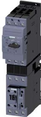
Load feeder fuseless, Direct-on-line starting 400 V AC, Size S2 28 ... 36 A 20 ... 33 V AC/DC screw terminal for installation on standard mounting rail (also fulfills type of coordination 1) Type of coordination 2, I<sub>q</sub> = 100 kA 1 NO+1 NC (contactor) with circuit (integrated)
