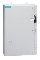
2-speed 3-phase motor starter Size 1 3/4 One winding consequent pole Constant or variable torque Solid-state overload relays Low SPD OLR range 10-40a High SPD OLR range 10-40a 110V 50HZ / 120V 60HZ coil Combination type 40AMP circuit breaker Encl NEMA type 4X 304 S-steel Water/dust tight noncorrosive
