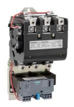
Non-reversing motor starter Size 2 1/2 Three phase full voltage Solid-state overload relay OLRelay amp range 25-100A 380-440/440-480V 50/60HZ coil Combination type No enclosure
