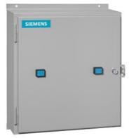
Duplex starter w/o alternator, Size 4, Three phase full voltage, Solid-state overload relay, OLR amp range 50-200A, 190-220/220-240V 50/60Hz coil, Non-combination type, Encl NEMA type 4X 304 S-Steel, Water/dust tight noncorrosive
