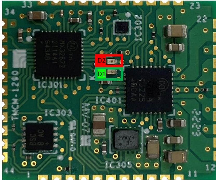
Figure 4: TMCM-1290 LEDs
