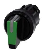
Selector switch, illuminable, 22 mm, round, plastic, green, selector switch, short, 3 switch positions I>O<II, momentary contact on the left, latching on the right, actuating angle  $2x45^{\circ}$ , 10:30h/12h/13:30h
