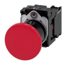
Mushroom pushbutton, 22 mm, round, plastic, red, 40mm, latching, pull-to-unlatch mechanism, with holder, 1 NC, screw terminal, with laser labeling, upper case and lower case, always upper case at beginning of line
