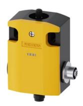
Basic switch without actuator head Metal enclosure, 56 mm wide ASIsafe integrated AS-i status: 1:F-IN1, 2: F-IN2 3:AS-i/FAULT Slow-action contacts 1 NC with M12 connector 4-pole Channel 1 to NC, Channel 2 to M12 socket on the right
